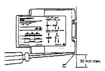
The H3DR can be mounted and dismounted with ease if a distance of 30 mm or more is kept between the H3DR and other equipment.
