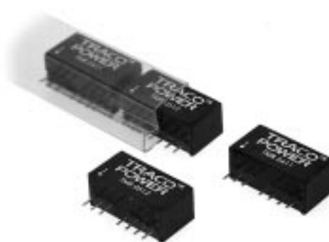
The TMR series is a range of miniature regulated 2 Watt DC/DC-converters in a SIL-package. Requiring only 2cm<sup>2</sup> board space they provide a state of art functionality. Wide 2:1 Input voltage range, 1000 VDC isolation voltage, external on/off control and a temperature range of -40°C – 85°C with no derating makes this converter suitable for many applications in telecommunication, control units and industrial equipments.
