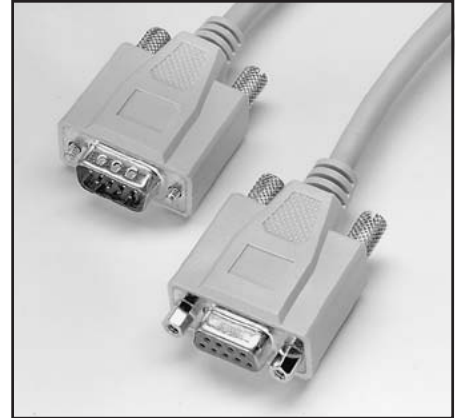
Model 7009-5 Shielded RS-232 Cable: 1.5m (5 ft) RS-232 cable with a male DB-9 connector at one end and a female DB-9 connector on the other end. Wired as a straight through, not as a null modem cable.
