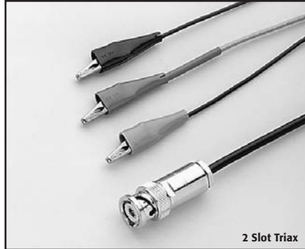
Model 6011 2-slot Triax Cable: 1.5m (5 ft) of triax cable (SC-22) terminated with a 2-slot triax plug on one end and three alligator clips on the other. Also available in 3m (10 ft) length (Model 6011-10).
