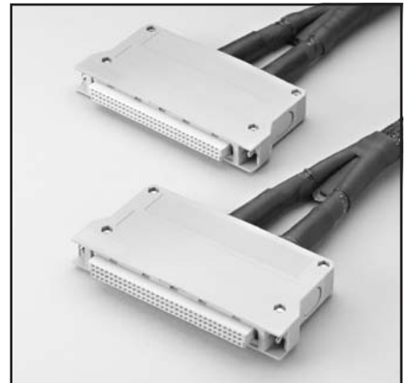
Model 7011-MTC-1: 1m (3.3 ft) mass terminated cable assembly for connection to 7011-C and other switching cards. The cable has 45 pairs with outer shield. The cable is terminated at each end with 96-pin female DIN connectors with strain relief. Also available in 2m (6.6 ft) length (Model 7011-MTC-2).
