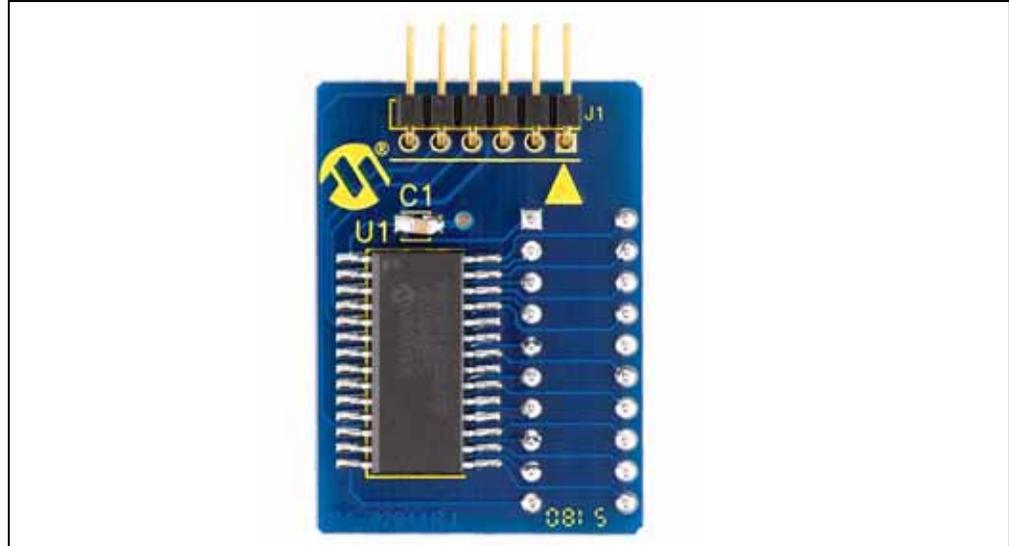
To use the debug header, simply remove the PIC18F14K50 mounted in the MCU socket (U2) on the Low Pin Count USB Development Board. Using a pin header (not included), connect the debug header into the MCU socket and connect the PICkit™ 2 programmer/debugger to the provided connection header.
