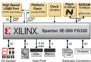
The on-board USB2 port provides power for the board, configures the FPGA and platform Flash, and allows high-speed data transfers with a PC. When driven from a notebook computer with the included USB2 cable, the Nexys-2 board can be used to build real circuits anytime, anywhere. Now everyone can own a powerful, state-of-the-art development system for less than the cost of a textbook!
