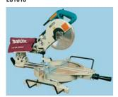
260 mm blade diameter slide compound mitre saw, bevel cuts  $45^{\circ}$  left or right. Features electric brake and soft start. Supplied with dust bag, vertical vice, TCT blade, holder set and triangular rule.
