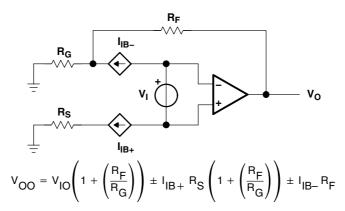
Figure 29. Output Offset Voltage Model
