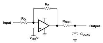
Figure 28. Driving a Capacitive Load
