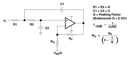
Figure 31. 2-Pole Low-Pass Sallen-Key Filter
