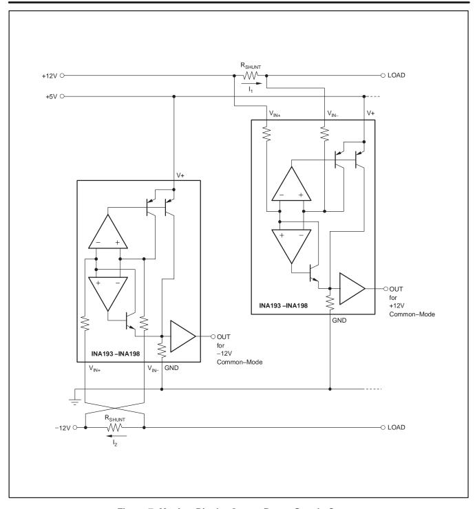
Figure 7. Monitor Bipolar Output Power-Supply Current
