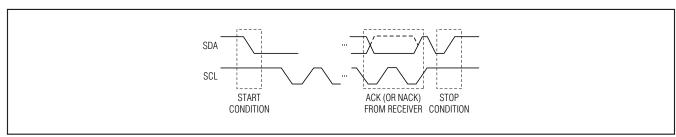
Figure 6. Start, Stop, and ACK Signals
