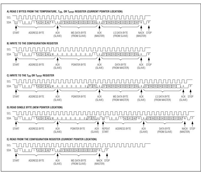
Figure 9. 2-Wire Interface Timing
