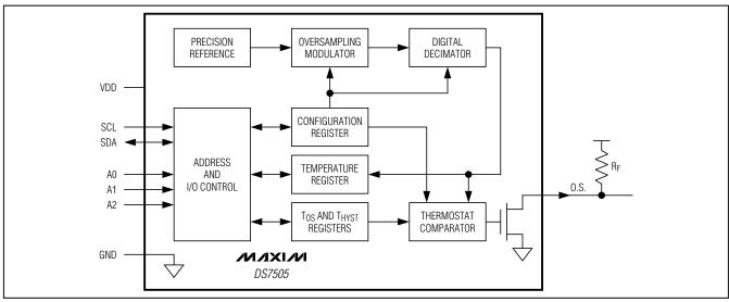
Figure 2. Block Diagram
