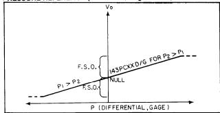
\*Reversing the pressure relationship of 141PC or 142PC will cause the output to saturate below null.
