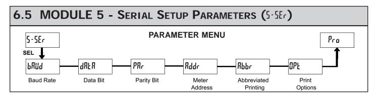
The Serial Setup Parameters are only active when one of the optional serial communication/programming cards is installed in the meter.
