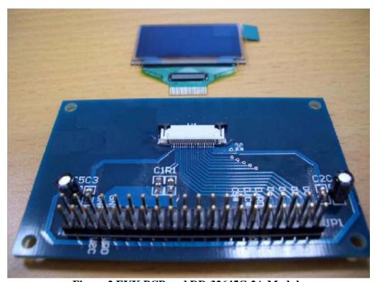
Figure 2 EVK PCB and DD-32645C-2A Module
