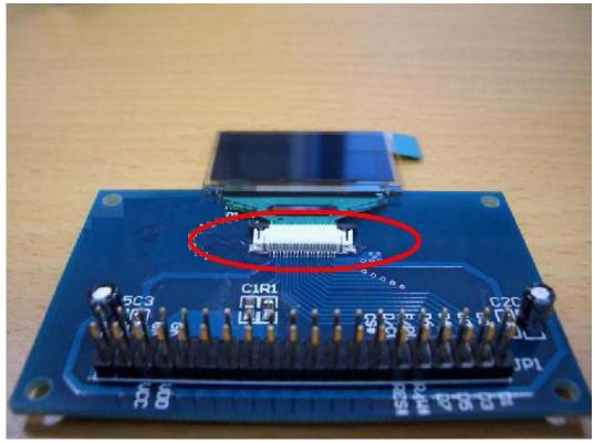
Figure 3 the DD-2832BE-2A and EVK assembled (Top view)
