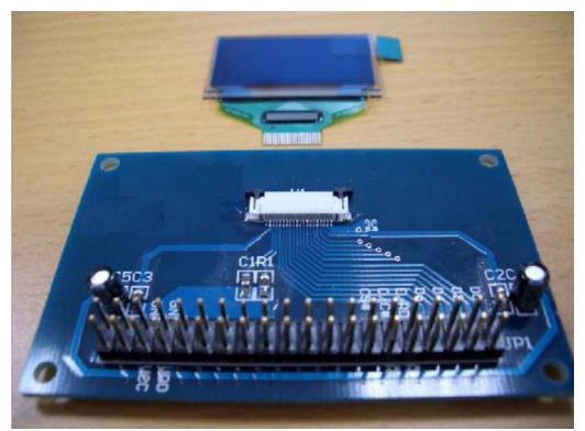
Figure 2 EVK PCB and DD-2864BY-2A Module
