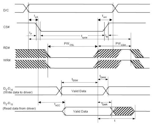
Figure 1 8080-series MPU parallel interface characteristics
