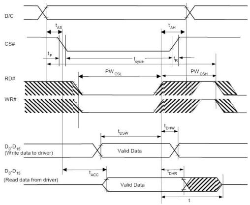
Figure 1 8080-series MPU parallel interface characteristics
