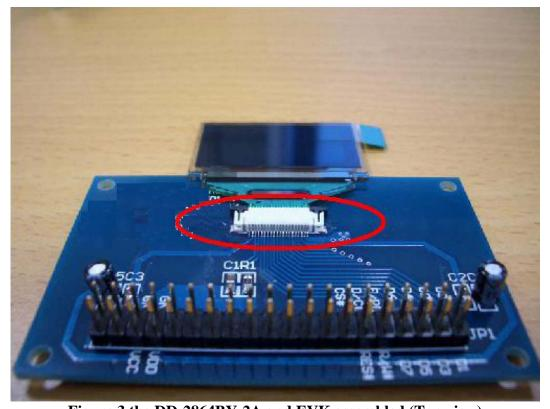
Figure 3 the DD-2864BY-2A and EVK assembled (Top view)
