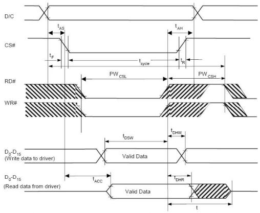
Figure 1 8080-series MPU parallel interface characteristics
