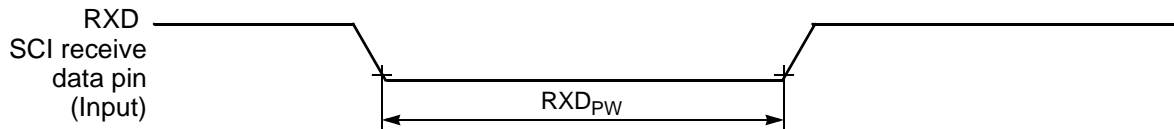
Figure 10-15 RXD Pulse Width
