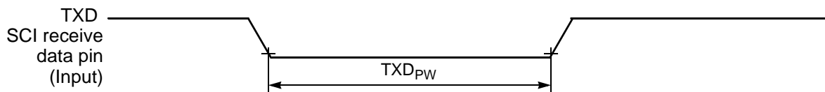
Figure 10-16 TXD Pulse Width
