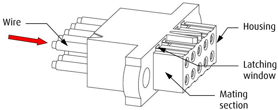
Push the contact and wire forward into the housing in the direction as shown, taking the load off of the contact latching feature on the contact.
