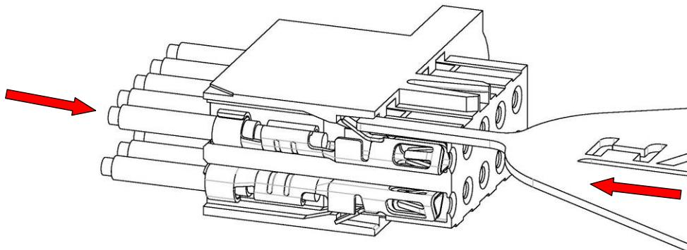
Slide the probe down the side of the mating section of the crimp housing, into the latching window of the crimp to be removed.
