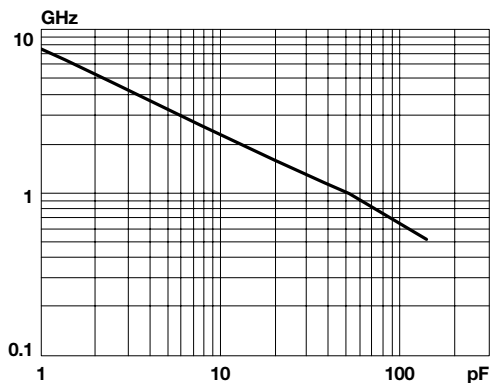
Typical Self Resonant Frequency vs. Capacitance Accu-F®/Accu-P® 0805
