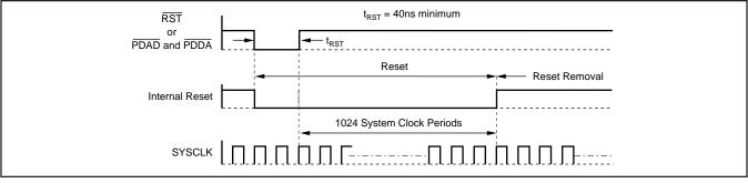
FIGURE 7. External Forced Reset Timing.
