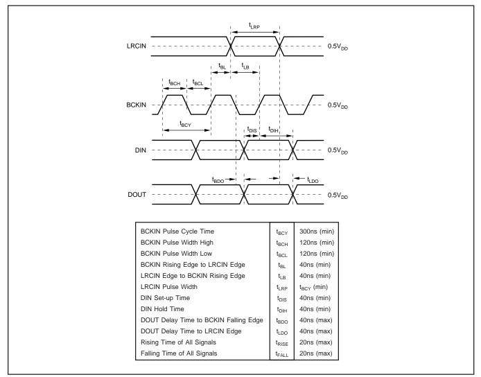
FIGURE 4. Audio Data Input/Output Timing.
