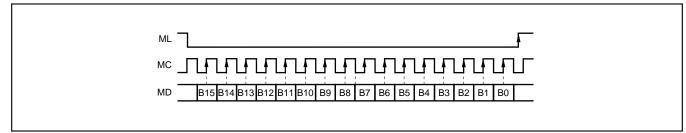
FIGURE 10. Control Data Input Format.
