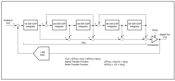
FIGURE 13. Simplified 5th-Order Delta-Sigma Modulator.
