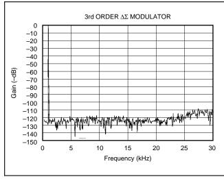
FIGURE 15. Quantization Noise Spectrum.
