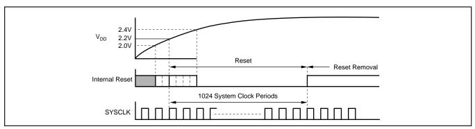
FIGURE 6. Internal Power-On Reset Timing.
