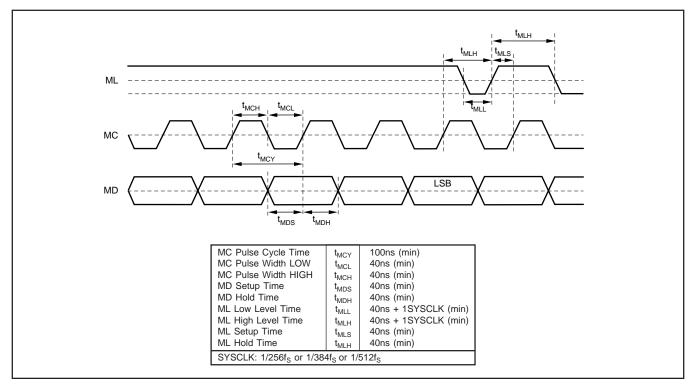
FIGURE 11. Control Data Input Timing.
