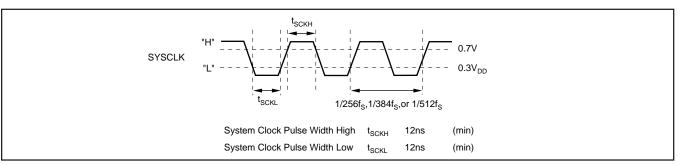
FIGURE 5. System Clock Timing.
