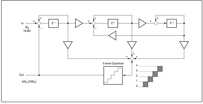
FIGURE 14. 5-Level Delta-Sigma Modulator Block Diagram.
