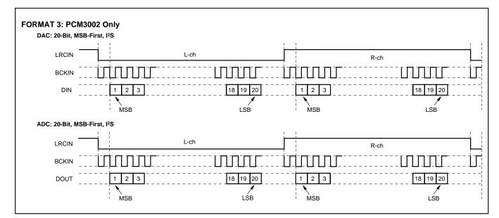
FIGURE 3. Audio Data Input/Output Format.
