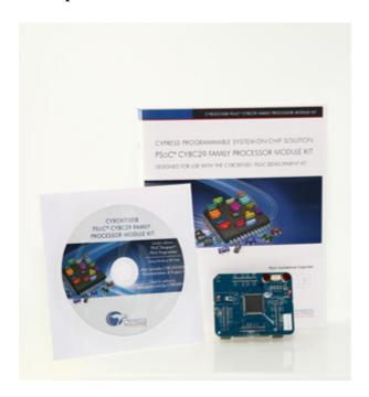
The PSoC® CY8C29 Family Processor Module is designed to evaluate and experiment with Cypress's PSoC 1 programmable system-on-chip design methodology and architecture. This processor module can be used in conjunction with the PSoC Development Kit (CY8CKIT-001) to create designs utilizing on-board DVK resources or compatible expansion boards. This kit provides you with an additional processor module to use with different projects.
