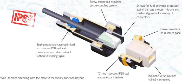
With Ethernet extending from the office to the factory floor and beyond into external environments, the demand for a secure connection for data applications is dramatically increasing.
