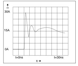
Figure 18. ESD Test Waveform for IEC1000-4-2
