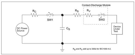
Figure 17. ESD Test Circuit for IEC1000-4-2
