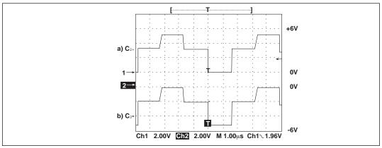
Figure 12. Charge Pump Waveforms
