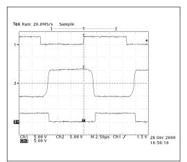
Figure 8. Loopback Test Circuit Result at 120kbps (All Drivers Fully Loaded)
