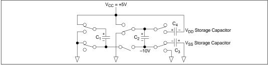
Figure 11. Charge Pump — Phase 2
