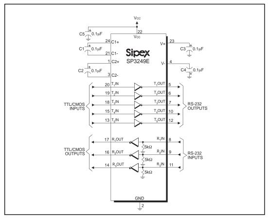
Figure 5. SP3249E Typical Operating Circuit
