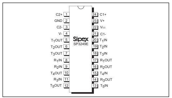
Figure 4. SP3249E Pinout Configuration
