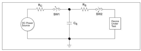
Figure 16. ESD Test Circuit for Human Body Model
