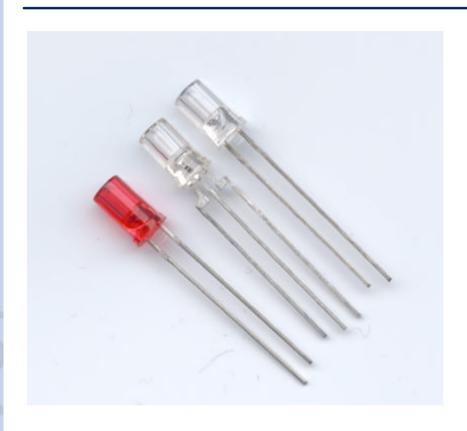
"Lochdiode" Transmitter and Receiver "Lochdiode" and "Verbinder"
