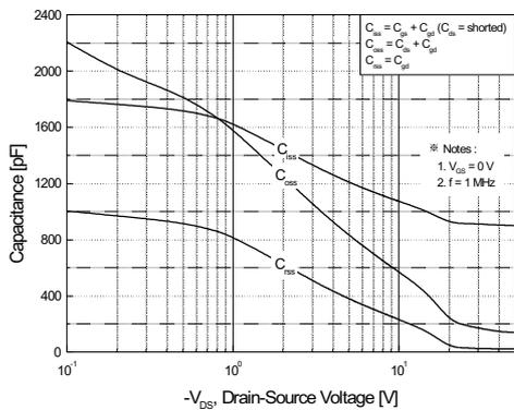
Figure 5. Capacitance Characteristics
