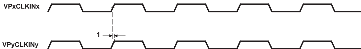
Figure 5-61. Video Port Dual-Display Sync Timing
