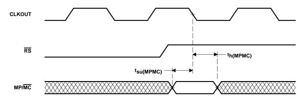
Figure 4–16. MP/MC Timing
