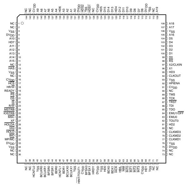
Figure 1-2. 144-Pin PGE Low-Profile Quad Flatpack (Top View)
