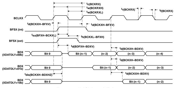
Figure 4–21. McBSP Transmit Timings
