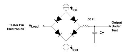
Where:  $I_{OL}$  = 1.5 mA (all outputs)  $I_{OH}$  = 300  $\mu$ A (all outputs)
