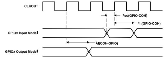
$<sup>^\</sup>dagger$  GPIOx refers to HD0, HD1, HD2, ...HD7, when the HD bus is configured for general-purpose input/output (I/O).
