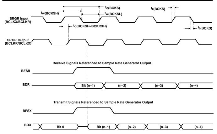
Figure 4-23. McBSP Sample Rate Generator Timings
