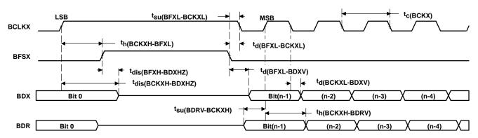
Figure 4-26. McBSP Timing as SPI Master or Slave: CLKSTP = 10b, CLKXP = 1
