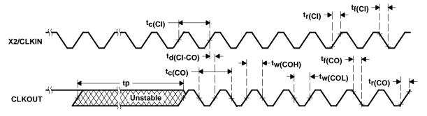
Figure 4–4. External Multiply-by-One Clock Timing
