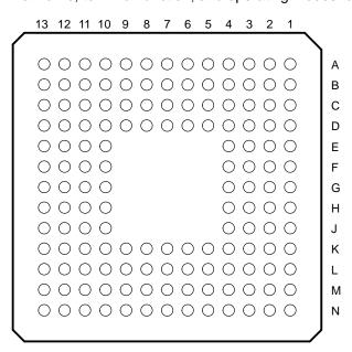
Figure 1–1. 144-Ball GGU MicroStar BGA™ (Bottom View)
