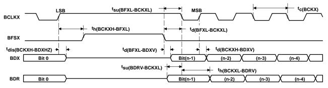
Figure 4-27. McBSP Timing as SPI Master or Slave: CLKSTP = 11b, CLKXP = 1
