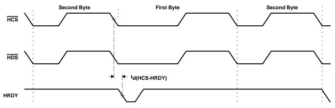
Figure 4–29. Using HCS to Control Accesses
