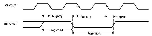
Figure 4–15. Interrupt Timing
