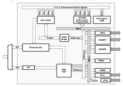
Figure 2-1. TMS320VC5401 Functional Block Diagram
