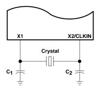
Figure 4-2. Internal Oscillator With External Crystal
