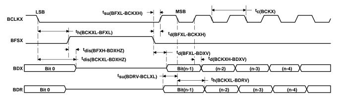
Figure 4–24. McBSP Timing as SPI Master or Slave: CLKSTP = 10b, CLKXP = 0
