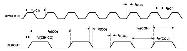
Figure 4-3. External Divide-by-Two Clock Timing
