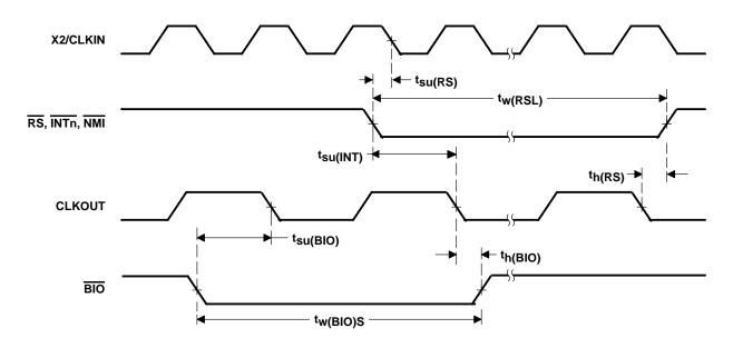
Figure 4–14. Reset and BIO Timings
