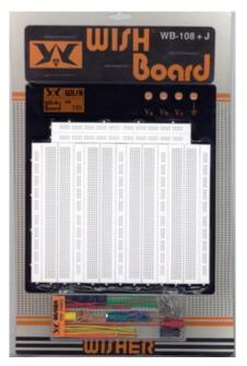
Material: high class ABS plastic, Dimension: 260 x 240 x 31 mm, Distribution strips: 7 Distribution holes: 700, Terminal strips: 4, Terminal holes: 2560,. Aluminium plate thick: 1.5, Knob post: 4, Foot pads: 5 With skin packing
