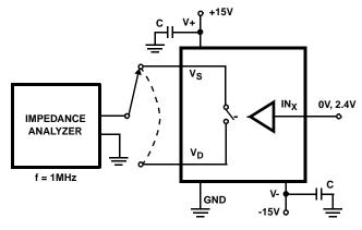
FIGURE 6. SOURCE/DRAIN CAPACITANCES TEST CIRCUIT
