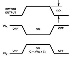
NOTE:  $\text{IN}_{X}$  dependent on switch configuration, input polarity determined by sense of switch.
