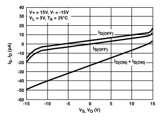
FIGURE 10. LEAKAGE CURRENTS vs ANALOG VOLTAGE
