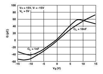
FIGURE 12. CHARGE INJECTION vs SOURCE VOLTAGE
