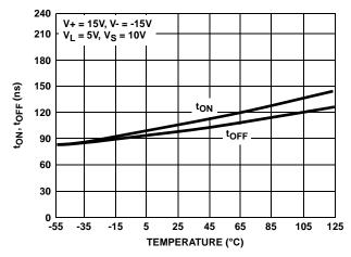
FIGURE 9. SWITCHING TIME vs TEMPERATURE
