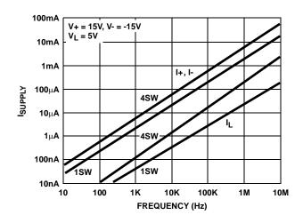
FIGURE 11. SUPPLY CURRENT vs INPUT SWITCHING FREQUENCY
