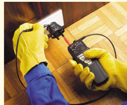
Used together, the C.A 751 + C.A 760 create a resistive phase-earth link for safely testing a 30 mA circuit breaker at 230 V AC.
