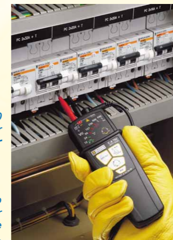
Used together, the C.A 751 + C.A 760 create a resistive phase-earth link for safely testing a 30 mA circuit breaker at 230 V AC.
