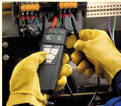
Phase rotation direction is defined by a TT, TN, or IT neutral system due to an innovative 2-wire method. This test operates on generator sets.
