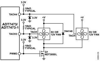
Figure 42. Fan with TACH Pull-Up to Vcc
