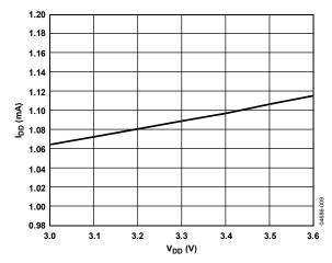
Figure 9. Normal IDD vs. Power Supply
