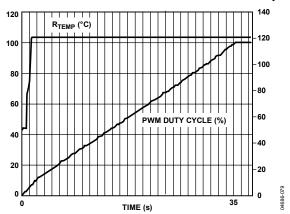
Figure 82. Enhanced Acoustics Mode with Ramp Rate = 1
