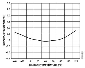
Figure 12. Internal Temperature Error vs. Temperature
