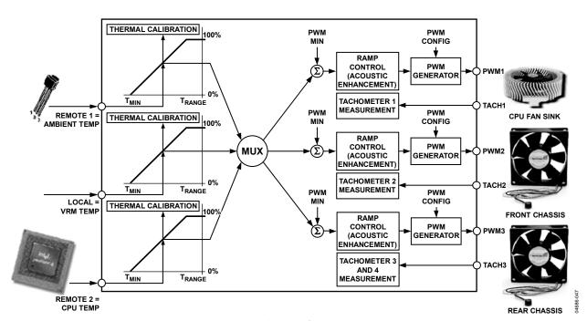
Figure 50. Hardware Configuration Example
