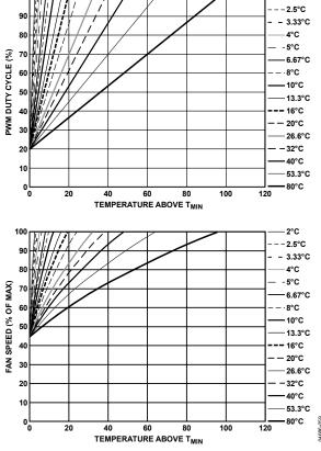
Figure 62. T<sub>RANGE</sub> and % Fan Speed Slopes with PWM<sub>MIN</sub> = 20%
