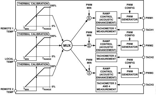
Figure 49. Automatic Fan Control Block Diagram
