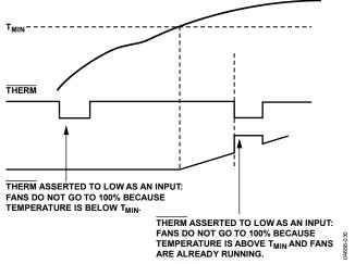
Figure 33. Asserting THERM Low as an Input in Automatic Fan Speed Control Mode
