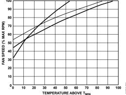
Figure 63.  $T_{RANGE}$  and % Fan Speed Slopes for VRM, Ambient, and **CPU Temperature Channels**
