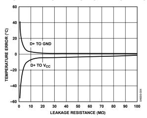
Figure 5. Remote Temperature Error vs. PCB Resistance
