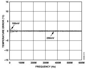
Figure 10. Internal Temperature Error vs. Frequency
