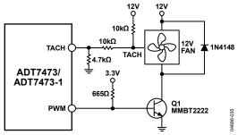
Figure 38. Driving a 3-Wire Fan Using an NPN Transistor
