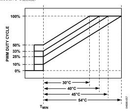
Figure 60. Increasing PWM<sub>MIN</sub> Changes Effective T<sub>RANGE</sub>
