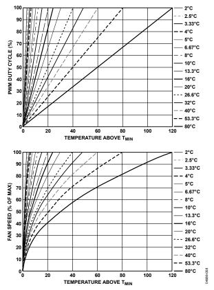
Figure 61. T<sub>RANGE</sub> vs. Actual Fan Speed Profile
