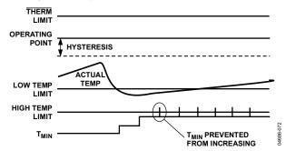
Figure 75. T<sub>MIN</sub> Adjustments Limited by the High Temperature Limit
