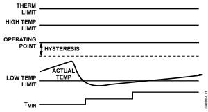
Figure 74. Increasing T<sub>MIN</sub> for Quieter Operation
