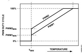
Figure 56. Operating Two Different Fans from a Single Temperature Channel
