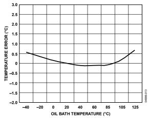
Figure 13. Remote Temperature Error vs. Temperature
