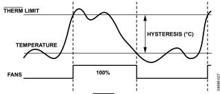
Figure 30. THERM Limit Operation
