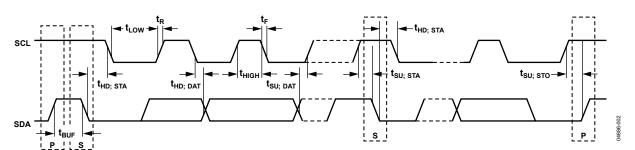
Figure 2. Serial Bus Timing Diagram
