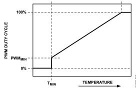
Figure 55. PWM<sub>MIN</sub> Determines Minimum PWM Duty Cycle
