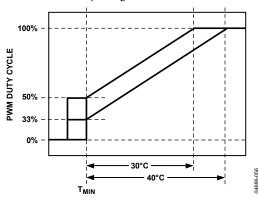
Figure 59. Adjusting PWM<sub>MIN</sub> Affects T<sub>RANGE</sub>
