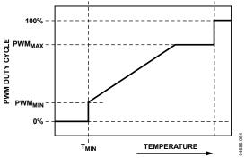
Figure 57. PWM<sub>MAX</sub> Determines Maximum PWM Duty Cycle Below the THERM Temperature Limit
