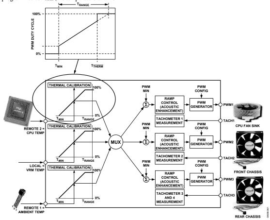
Figure 64. How  $T_{\overline{THERM}}$  Relates to Automatic Fan Control
