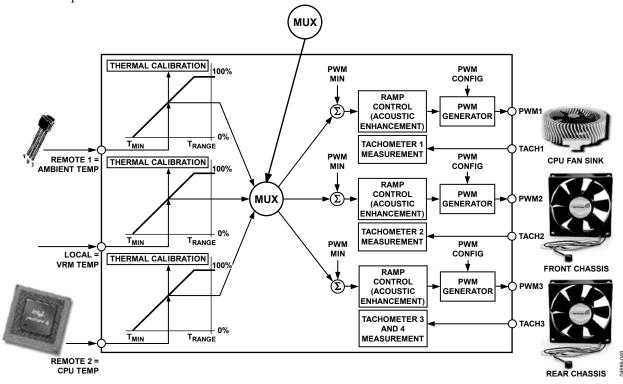
Figure 52. Assigning Temperature Channels to Fan Channels
