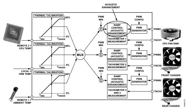
Figure 76. Acoustic Enhancement Smoothes Fan Speed Variations Under Automatic Fan Speed Control
