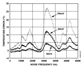
Figure 7. Remote Temperature Error vs. Common-Mode Noise Frequency
