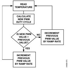
Figure 78. Enhanced Acoustics Algorithm
