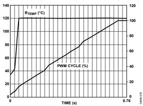
Figure 79. Enhanced Acoustics Mode with Ramp Rate = 48
