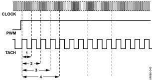
Figure 46. Fan Speed Measurement
