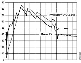
Figure 83. How Fan Reacts to Temperature Variation in Enhanced Acoustics Mode
