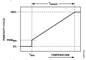
Figure 58.  $T_{RANGE}$  Parameter Affects Cooling Slope
