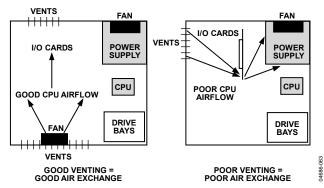
Figure 66. Chassis Airflow Issues
