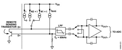
Figure 26. Signal Conditioning for Remote Diode Temperature Sensors
