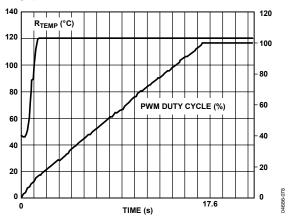
Figure 81. Enhanced Acoustics Mode with Ramp Rate = 2
