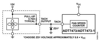
Figure 43. Fan with TACH Pull-Up to Voltage > 3.6 V Clamped with Zener Diode
