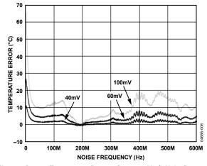
Figure 8. Remote Temperature Error vs. Common-Mode Noise Frequency
