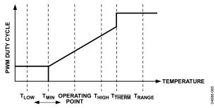
Figure 68. Dynamic T<sub>MIN</sub> Control Loop
