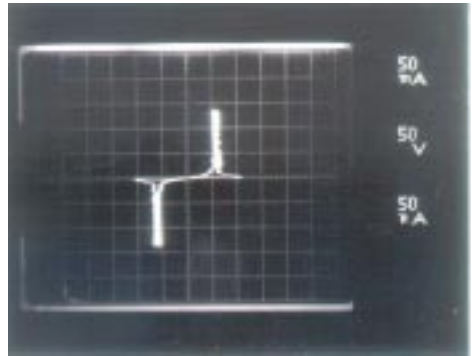
Figure 2 Current vs Voltage Characteristics for 8W Linear Fluorescent Tube.
