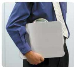
**This balance is especially suitable for mobile use** thanks to its battery supply and its flat construction
