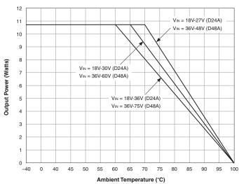
D24A and D48A Temperature Derating for 3.3V Output Models
