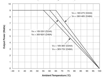
D24A and D48A Temperature Derating for 1.8V Output Models
