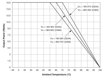
D24A and D48A Temperature Derating for 1.5V Output Models
