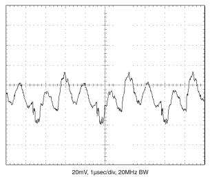
Output Ripple and Noise (PARD) (VIN = nominal, Vout = 12V @ 1.25A, two ext. 0.47 $\mu$ F output capacitors.)
