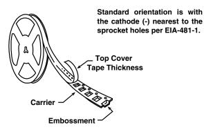
Tape and Reel Specifications: All case codes are available on plastic embossed tape per EIA-481-1. Standard reel diameter is 13" [330 mm]. 7" [178 mm] reels are available.
