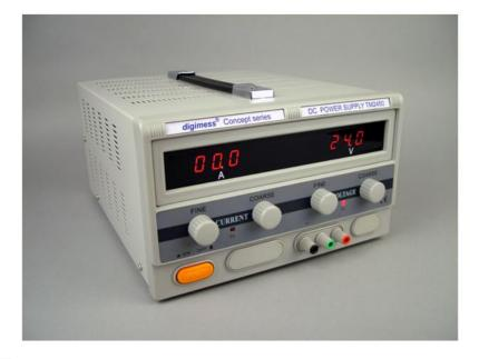
The *digimess*® TM series is a range of general purpose switch mode power supply units featuring high output currents. All models can operate in either constant voltage or constant current modes and feature large red LED displays for ease of viewing. The switch mode design results in small and light weight units compared to their linear equivalents. All units are supplied with mains leads and operating manuals.
