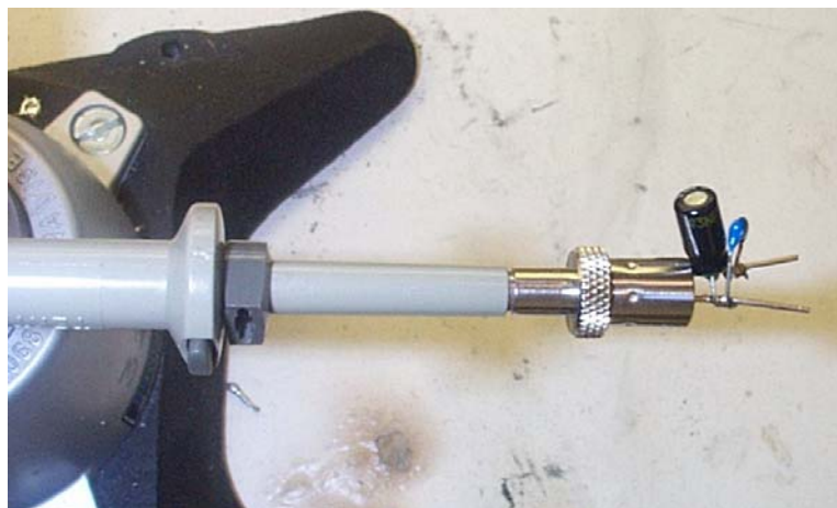
Figure 32 – Oscilloscope Probe with Probe Master 5125BA BNC Adapter. (Modified with wires for probe ground for ripple measurement, and two parallel decoupling capacitors added)
