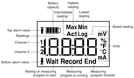
The following units are shown in the **175 - S2** data logger display: mV, %, °F, °C and mA. No unit appears in the display if other units are selected in ComSoft. The selected unit is displayed in the readings if the saved data is imported to ComSoft.
