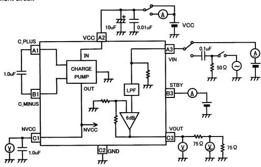
\* Measurement circuit is intended for shipment inspections, and differs from application circuit.
