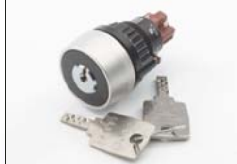
Keylock switch, 2 position, raised, gold over silver contacts, solder terminals, snap-action
