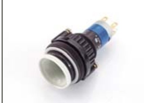
Illuminated pushbutton actuator for raised and flush mount, black plastic, plug-in terminal, snap-action, gold over silver contacts
