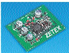
Evaluation board supporting the Zetex PWM DC-DC controllers.
