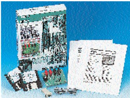
The DS2437K allows for evaluation, software development and prototyping of the DS2437 Smart Battery Monitor. The circuit board interfaces to a PC via an adapter and the software runs under Windows '95 with a select mode to run in demonstration or design mode. To operate, select current rate via sense resistors set by jump connectors, attach a voltage source and test drive the on-board DS2437 or program an additional device on the provided socket for prototyping.
