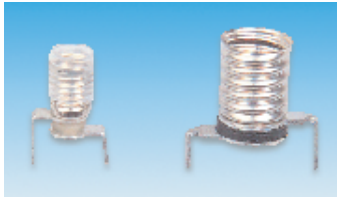
LES L = 17.1 (overall) Pin dia. = 1.42 MES L = 19.1 (overall) Pin dia. = 2.0
