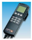
An electronic combustion gas analyser for the control of burner efficiencies and the measurement of environmental emissions from boiler plants. Under the 1990 Environmen-tal Protection Act (EPA) there is increasing legislative control of a wide range of new and existing industrial and commercial process-
