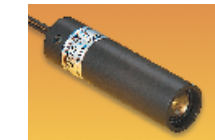
678-960 Body dia. = 14, L = 50 Outer thread = M6 0.75, L = 9.5
