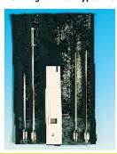
A pen type pocket sized 3 digit LCD thermometer with a wide measuring range, -160°C to +850°C. A range of screw-in stainless steel type K thermocouple probes is available for general purpose/immersion, and surface measurement applications.
