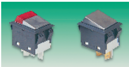
Illuminated Non-illuminated Bezel = 35.4 27.4, Depth = 33.25, Panel cut-out = 34.5 23.5, Tabs = 6.3
