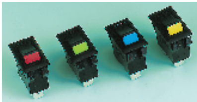
Bezel = 31 17, Depth = 30.3, Tabs = 6.3 0.8 Cut out: 1mm panel (min) 28.6 14 -3mm panel (max) 28.8 14
