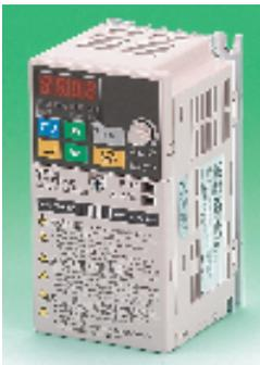
The 3G3MV inverter is an extremely compact, easy to use open loop vector control inverter and has versions available in single phase 240V AC, three phase 200V and three phase 400Vac up to 4kW
